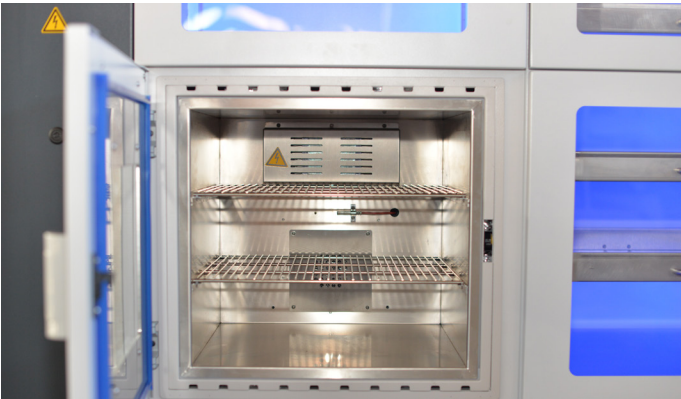
Tempering oven with automatic locking, adjustable 125°-140°C
