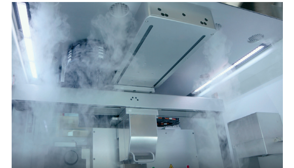
Controllable microenvironments in the process cabinet
