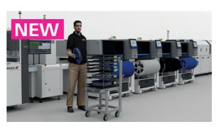
The mobile material transport system Pick-by-Light-mobile represents the interface to the line replenishment of the placement systems. The machine can pick up a filled reel magazine, presents it to the operator and visualizes the next required SMD component reel via the LED light function of the smart labels.
