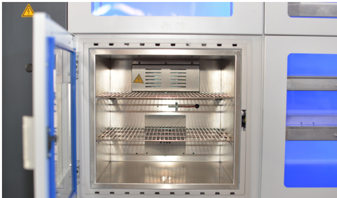
Tempering oven with automatic locking, adjustable 125°-140°C
