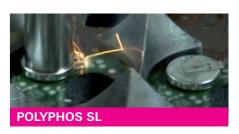
Selective laser reflow of temperaturesensitive components.
