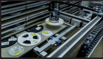
The quantities and states of all materials on the entire shop floor are clearly documented in the PULSE PRO module "Material". All component reels, trays and PCBs are managed on the basis of Unique ID (UID) and the replenishment of material is controlled autonomously, which reduces the operator's workload. Furthermore, the floor
