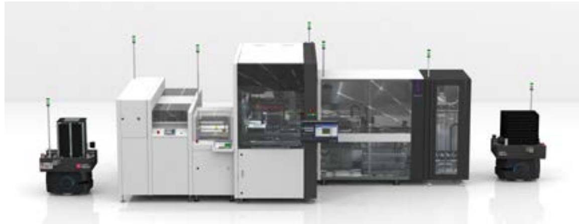
Fully Automated DIVISIO Production Island with PARIO 800 for Part Unloading
